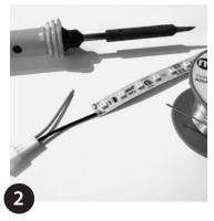
Carefully solder prepared cable to marked solder pads. Minimise contact time to avoid excessive heating of the strip.
